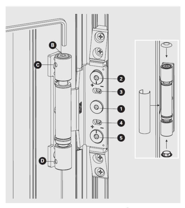
Horizontal adjustment: unscrew by three turns, screw 1. Tighten or loosen alternately screws 3 and 4 with a 4 mm Allen Key. Tighten screw 1. Adjustment ± 3mm.
